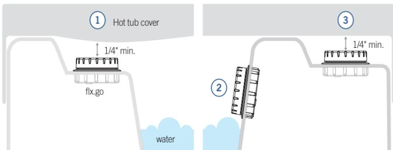
The flx.go can be installed facing inside the hot tub either horizontally (1) or vertically (2). When installed facing in, the flx.go must be mounted **above the water line**. It can also be installed facing out like standard keypads (3). Proper clearance (1/4" min.) needs to be planned to make sure the hot tub cover does not come into contact with the flx.go.
