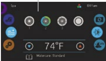
Variable speed pump icon on
