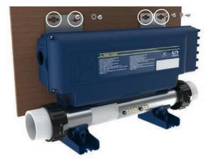
Use 2 standard 2" x 4" or 2" x 6" wall studs, spaced 17-inch from center to center to fix the spa pack.
