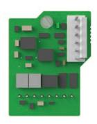
Optional extension communication board for in.temp support. Can be ordered directly as an option on in.ye or separately
