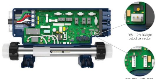
P63; P64 - LEDs RGB output connectors
