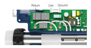
The heat.wav heater is factory configured for 240 V / 4 kW, but it can be converted to a dedicated 120 V / 1 kW by simply adding a cable connection. (120 V conversion is available on North American in.ye-3 models only).
