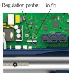
in.ye systems come with a high performance heat.wav heater. With no pressure switch, it features in.flo integrated dry-fire protection.
