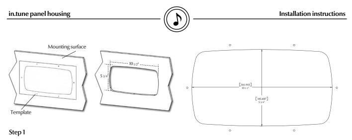
Using the drilling template supplied with the unit, determine the mounting location and then stick the template on the location.
