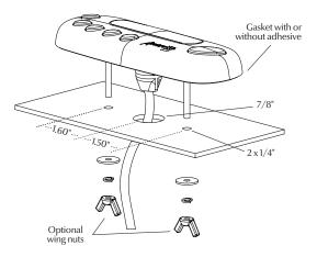
To install the in.k400, the user must cut out one 7/8" diameter hole for the cable (see illustration).
