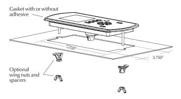
To install the in.k600<sup>™</sup> low profile, use the drilling template provided in this section. Determine the mounting location and stick the template on chosen location. The user must cut out a rectangular shape opening of 7.250" by 3.750" according to the template (see illustration).
