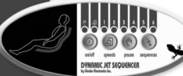
Your Dynamic Jet Sequencer controls 4 jet sets in your spa's "hot seat". This **Quick Reference Card** provides a quick overview of your jet sequencer's main functions and the operations accessible with your DJS-1 keypad.
