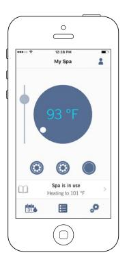
Touch the centered widget to reveal the temperature control bar.
