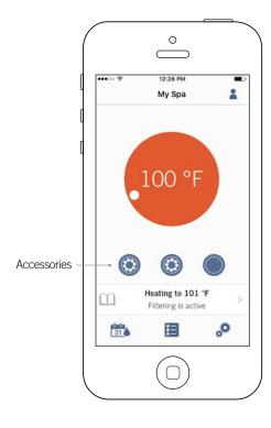
According to your customer's spa control system configuration, you can start or stop an accessory by simply touching the associated icon. The icon will become animated when the accessory is on. Simply press on the icon to start or stop the accessory. If the accessory has more than one speed, press the button until the desired speed is reached.
